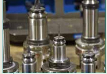
REGO-FIX powRgrip toolholders provide Northeast Tire Mold with extremely low TIR, which is mandatory for the shop's use of very small cutters at lengths of up to 15 times cutter diameter.
