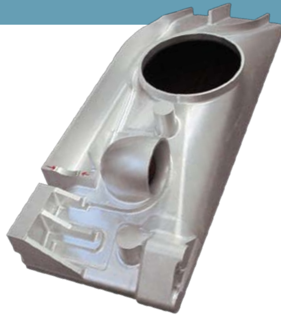
A five-piece weldment part that MAC Machine produces is difficult to machine because of the complex geometries of the unit.
