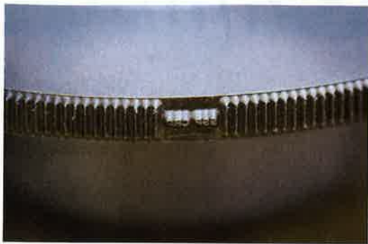
The smallest marking dies the shop makes feature letters measuring only 0.62-inch high.
